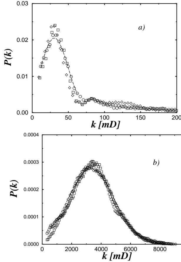
**Fig. 3.** Normalized permeability distributions for the Sample Ho corresponding to (a) low permeability zone, and (b) high permeability zone. In both figures we plot the distributions corresponding to three different faces of the sample. The distributions are fitted by Gaussian functions. We notice the large difference in the mean value of the permeability between the low and high permeability zones.
