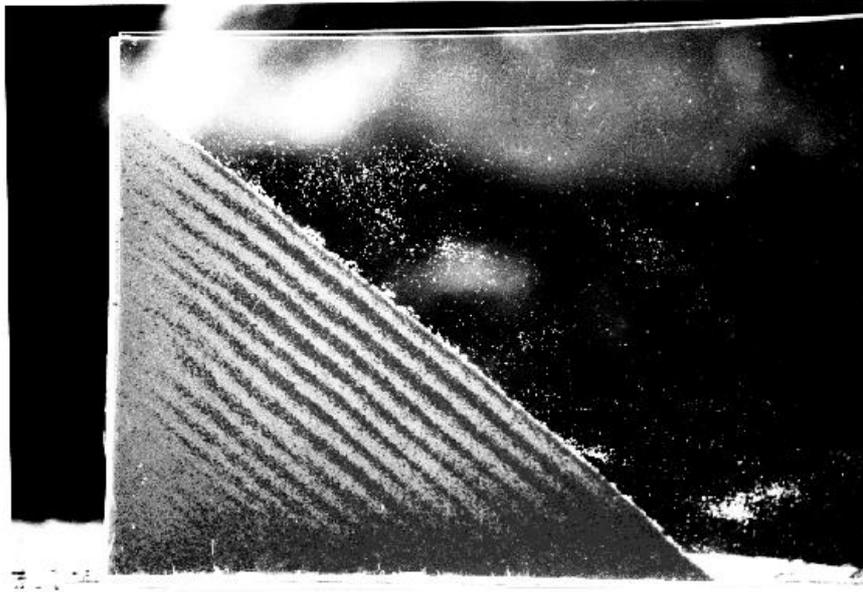
**Fig. 2.** Photograph of the experimental sandpile showing the periodic layers.
