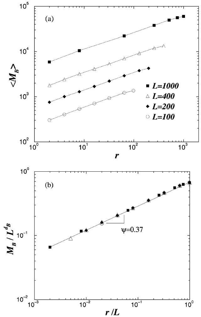
FIG. 2. (a) Log-log plot of the average backbone mass  $\langle M_B \rangle$  vs  $r$  for four different values of  $L$ . (b) Data from Fig. 2(a) collapsed with the use of the scaling form proposed in Eq. (3). The error on  $\psi$  is typically 0.02.
