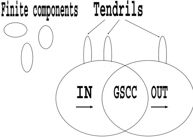
**Fig. 3.1.** Structure of a general directed graph
