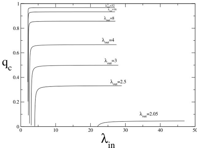
**Fig. 3.3.** The critical concentration as a function of  $\lambda_{in}$  and  $\lambda_{out}$ . Notice the steep change at the boundaries of the transition between the resilient and non resilient regimes. This plot was obtained for  $A = 0.05$
