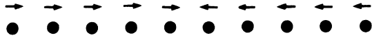
FIG. 1. The configuration with oriented fields which leads to the largest survival among all possible configurations. The arrows indicate the preferred direction for particle movement. This direction is characterized by a probability P=(1+E)/2 .
