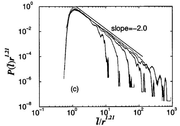
FIG. 2. (a) Log-log plot of traveling distance distribution  $P(\bar{\ell})$  for  $r=4, 8, 16, 32, 64,$  and  $128$ . (b) Log-log plot of the most probable traveling length versus  $r$ . A linear fit yields  $d_{\bar{\ell}} = 1.21 \pm 0.02$ . (c) The data obtained by rescaling the traveling length with its characteristic length  $\bar{\ell}^* \sim r^{1.21}$ . A fit of the power-law regime gives  $g_{\bar{\ell}} = 2.0 \pm 0.05$ .
